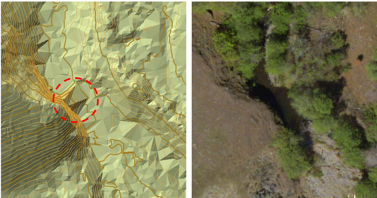
Figure D2. Example of an artificial projection into stream channel by terrain data artifact (left) , in this case extending 17' into a channel with 24' toe width. Aerial photograph of same site (right).
