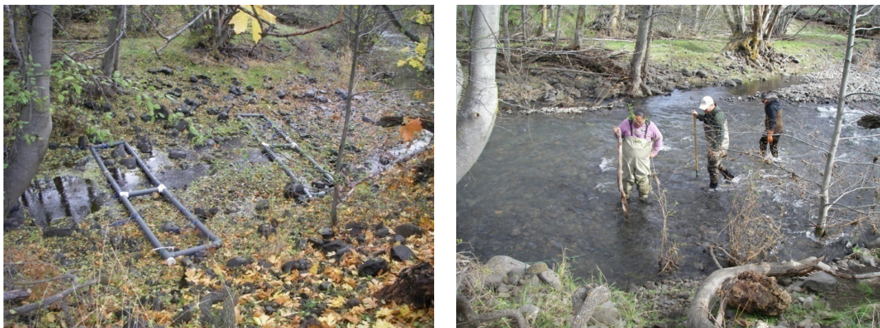
Figure 79. PIT-tag array near mouth of Squaw Cr before (left) and immediately after (right, buried) 2012 peak flow (~Q3). Photos courtesy of B. Allen, USGS.
