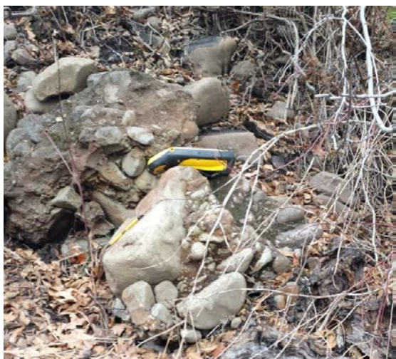
Figure 70. Exposures of indurated sediments were observed locally throughout the field-surveyed area, generally exhibiting greater erosion resistance and frequently associated with groundwater expression.
