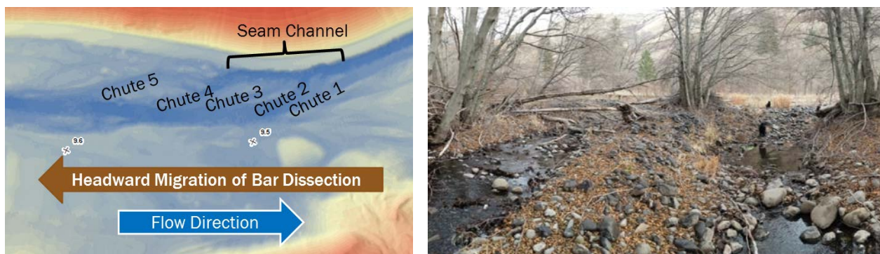
Figure 75. Schematic showing development of high-relief diagonal bar (left) and upstream view of chutes (right).
