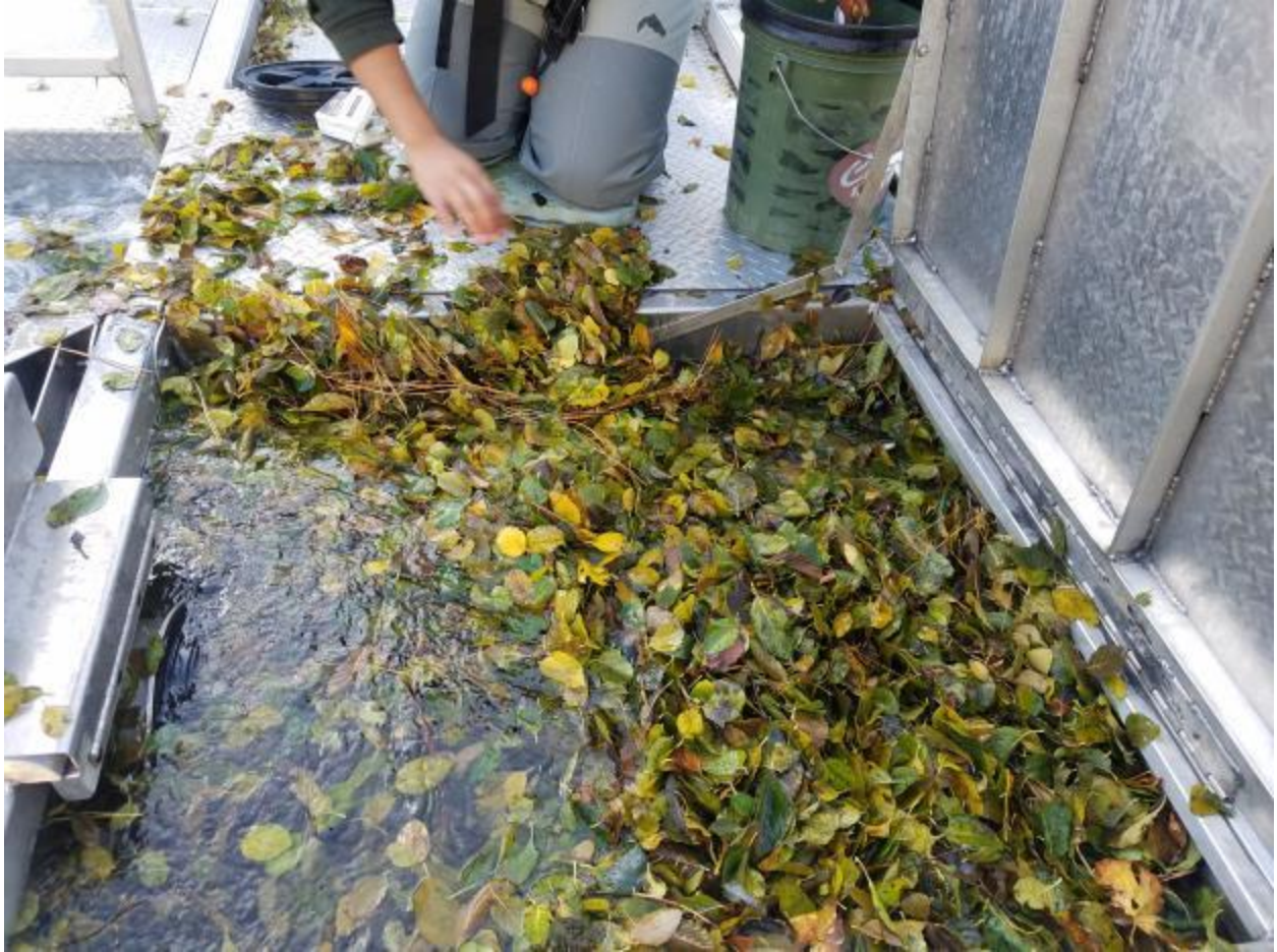
Appendix D. Photo documenting debris accumulation in live-box after a high debris loading event during elevated spring flows at the rotary screw trap in the Klickitat River, WA.
