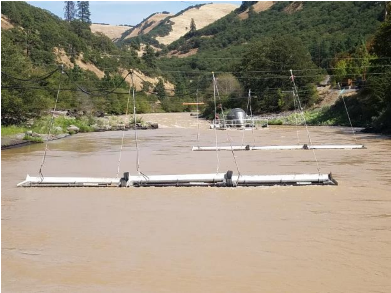
Figure 3. Photos of the rotary screw trap and floating PIT tag interrogation array at river kilometer 4.5. Photo descriptions starting at top left and proceeding clockwise: aerial view looking north to south, aerial view south to north, and downstream to upstream view at the channel level (aerial photos by David Lindley).
