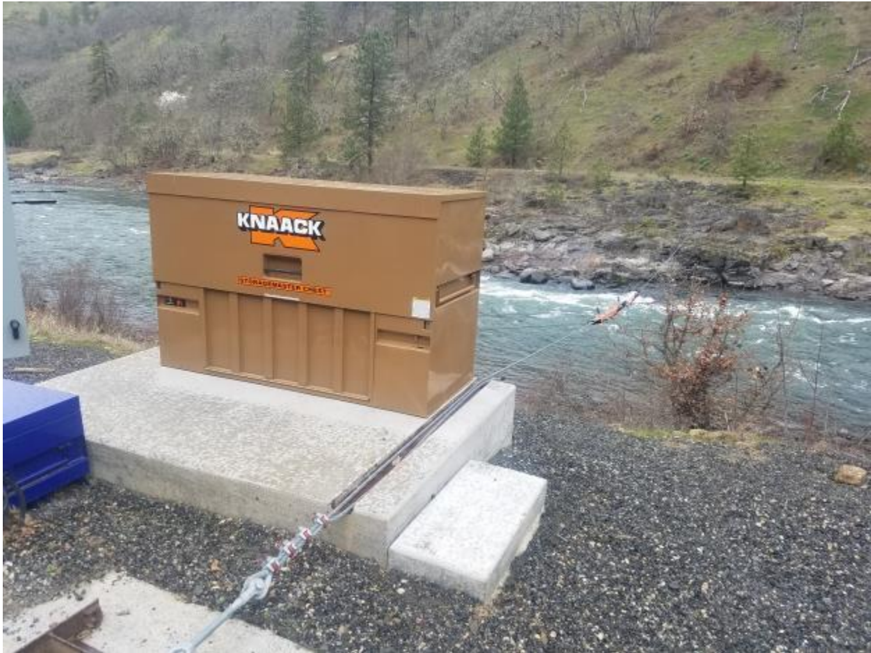
Appendix A. Photo of electronically powered winch used to laterally move the rotary screw trap across the river channel. The winch is located on the east bank at river kilometer 4.5, Klickitat River, WA.
